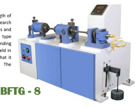
A complete cycle of reversed stresses in all fibers of the specimen is produced during each revolution. The bending moment is applied with a lever system and can be easily changed by moving weight over the lever. Total number of revolutions at which the specimen fails is recorded by a Digital Counter. An interlocking system puts off the motor at specimen failure, Machine meets requirements of IS 5075-1959.
